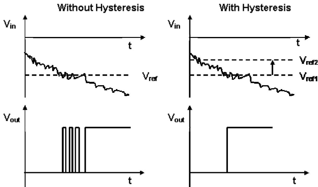
Figure 9: The input and output voltage of the comparator as a function of time, with and without hysteresis caused by positive feedback. Smaller feedback resistance  $R$  will cause a larger shift of  $V_{ref}$  when the output switches initially.
