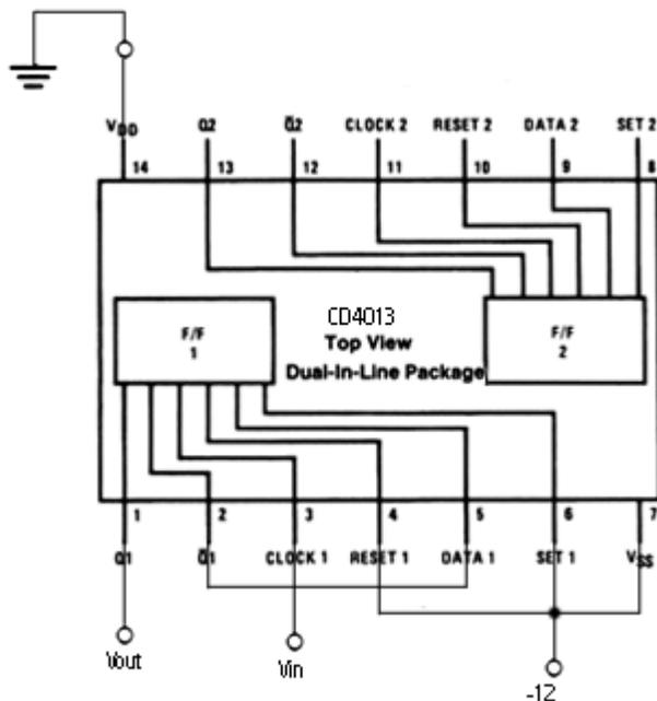
Figure 10: Flip-flop wiring diagram. The input comes from the comparator
