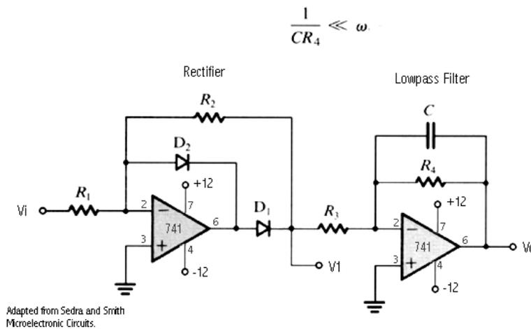
Figure 7: Rectifier and Lowpass Filter
