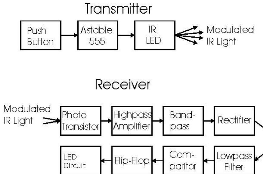
Figure 1: Block diagram of the IR transmitter and receiver
