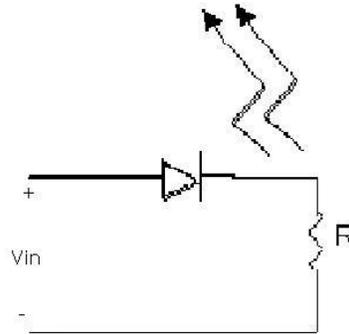
Figure 11: LED Circuit
